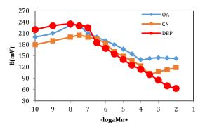
Fig. 1 Calibration curve of fluoride selective electrode with different plasticizers
